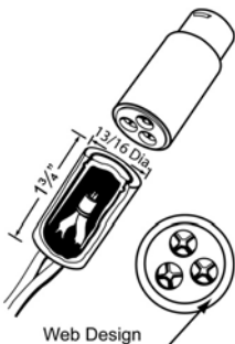
Web Design allows easy insertion of wire, expands to appropriate wire size and seals any unused holes to prevent sealant run out
