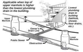
Spears<sup>®</sup> Backwater Valve is additionally rated to 100 psi for use in balancing multi-level systems such as tank storage and ponds.
