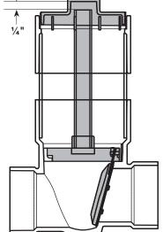
**STEP 5** Cement flapper assembly to one end of the internal extension pipe.
