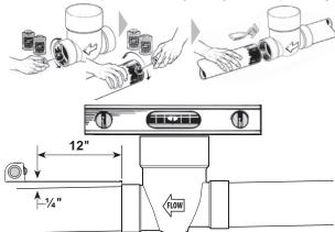
CAUTION: Valve must be installed horizontally with proper direction of flow. Do not install upside down.
